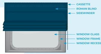
When installing into the recess, make sure the blind isn't installed too close to the window and be aware of any obstructions such as window handles that need to be avoided.
